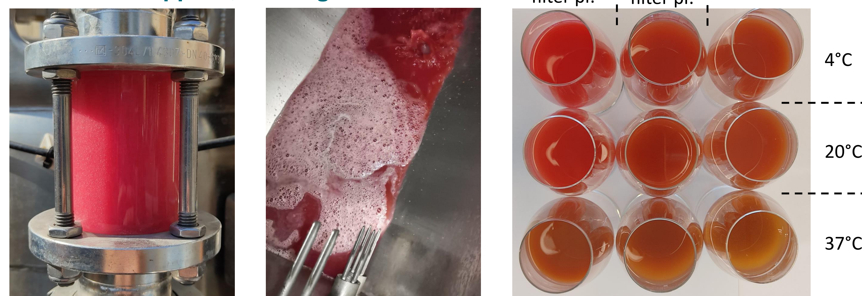
Fig. 2: Sight glass spiral filter press (l.), juice basin horizontal filter press (m.), juices after 12 month of storage (r.).
